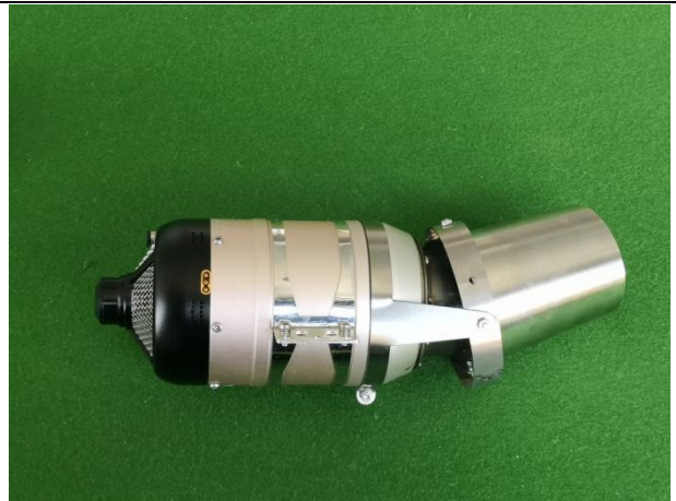
vector thrust up/down 40 degree
